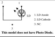
Initial Electrical/Optical Characteristics  $(Tc=25^{\circ}C)$ Condition Symbol Item Min Max Unit Typ. **Optical Output Power** Po 0.75 1.00 If=1.0A \_ W Dominant Wavelength If=1.0A λd 440 455 \_ nm CW Threshold Current Ith 100 300 mA Slope Efficiency CW 0.8 \_ 1.8 W/A η If=1.0A V **Operating Voltage** Vop 4.0 6.0 \_ θ// 5 12 25 Beam Divergence deg. If=1.0A Full Angle  $(1/e^2)$ 30 40 50  $\theta \perp$ deg. **Emission Point** If=1.0A deg.  $\Delta \theta \perp$ -5.0 5.0 Accuracy
